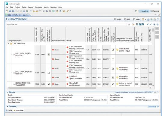
Leading automotive companies use medini analyze to support best-practice workflows that graphically link specific areas of the semiconductor design to key functions within the electronics architecture. This allows engineers to analyze and address potential failure modes as they verify the functional safety of semiconductor components.
