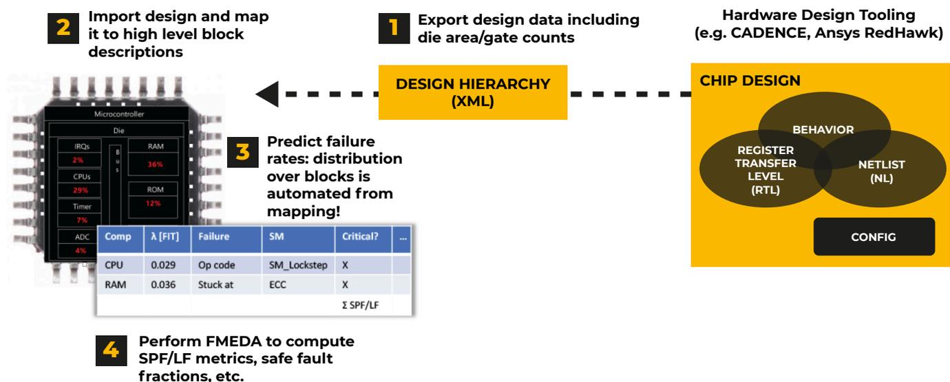
Via a step-by-step, automated process, medini analyze enables automotive engineers to perform failure modes, effects and diagnostic analysis (FMEDA) for all semiconductor components in a rapid, cost-effective manner.
